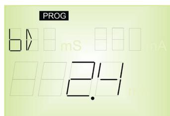
Repeatedly press the **td** button to change the baud rate, increasing the value of a digits on the central area of the screen.
